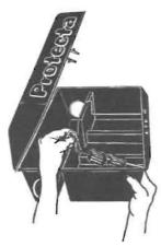
2 Insert that end into the circular groove inside the front wall of the station.
