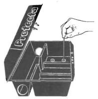
1 Insert either end of the PROTECTA Vertical Bait Securing Rod into one of the holes in the floor of the baiting areas.
