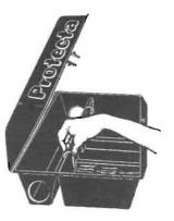
Insert the hooked end of the rod into the hole on top of the baffling and push down to secure.
